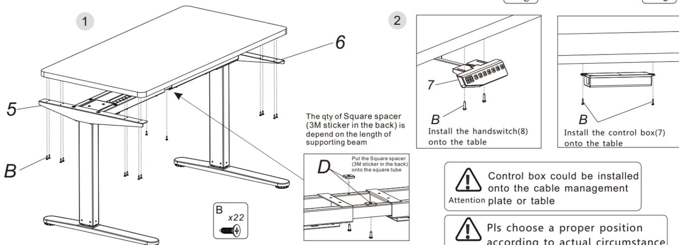
**Attention** Control box could be installed onto the cable management plate or table
