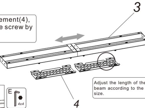
Use 4\*4 wrench (E) to untighten 8 screw on the back of supporting beam (3) in case you need to adjust the length.
