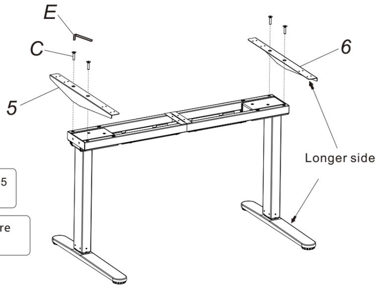
Install supporting plate(5)(6), use 5\*5 wrench(E) to tighten the screws(C)
