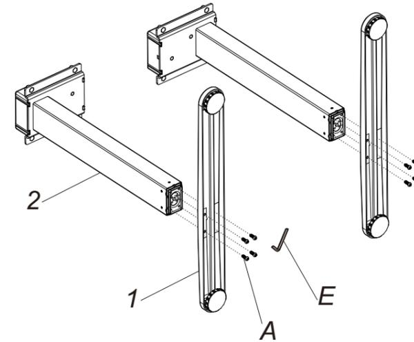
Install 1 & 2 together, use 4\*4wrench(E) to tighten the screws(A).
