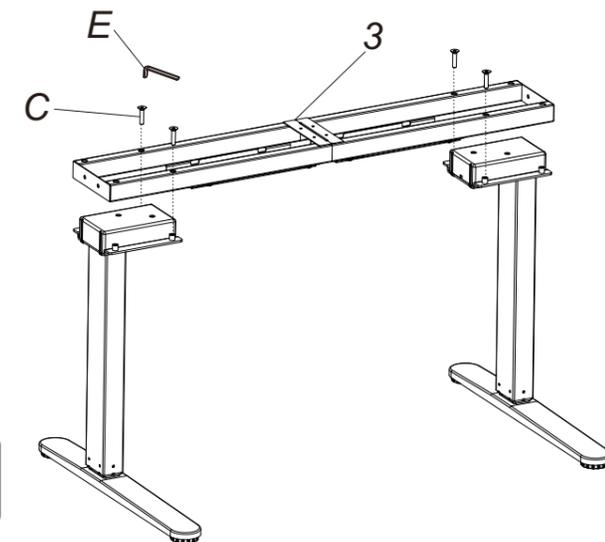
Install the supporting beam(3) use 5\*5 wrench(E) to tighten the screws(C).
